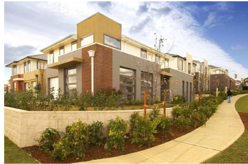
Using 'breaks' in levels to identify public and private - 'What's mine and what belongs to the public'
