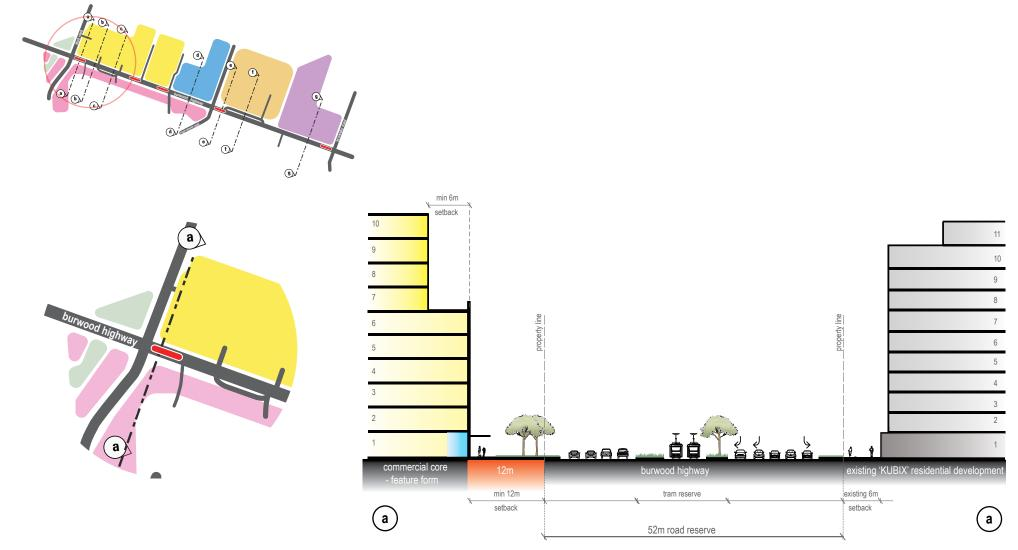
Figure 7. Section AA - Commercial Core
