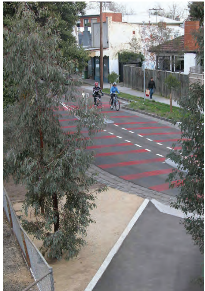
Safe street in Footscray. Small speed humps reduce speed
