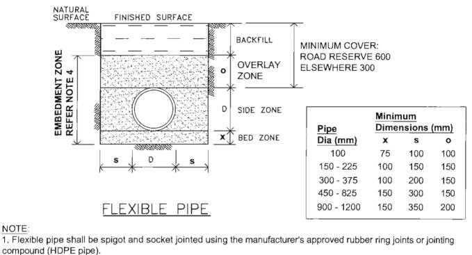
2.UPVC pipes shall be Class SH (sewer quality), 100 minimum diameter.
