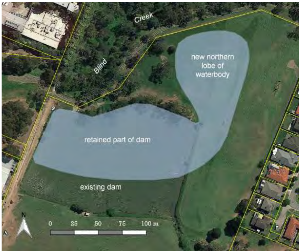
Figure 5. A concept plan for a new open waterbody (in semi-transparent blue) that retains the dam's existing north shore and would leave the vegetation on that shore out of bounds to the public.
