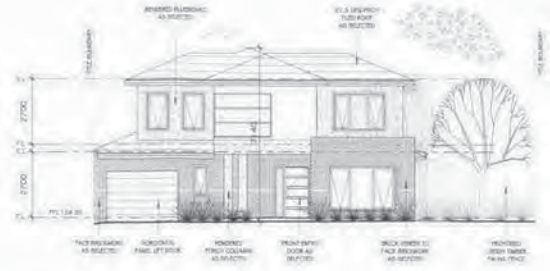
2 EAST ELEVATION D3 1:100
