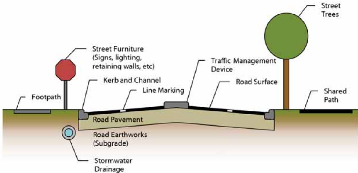
Figure 4 Typical Assets in the Road Reserve
