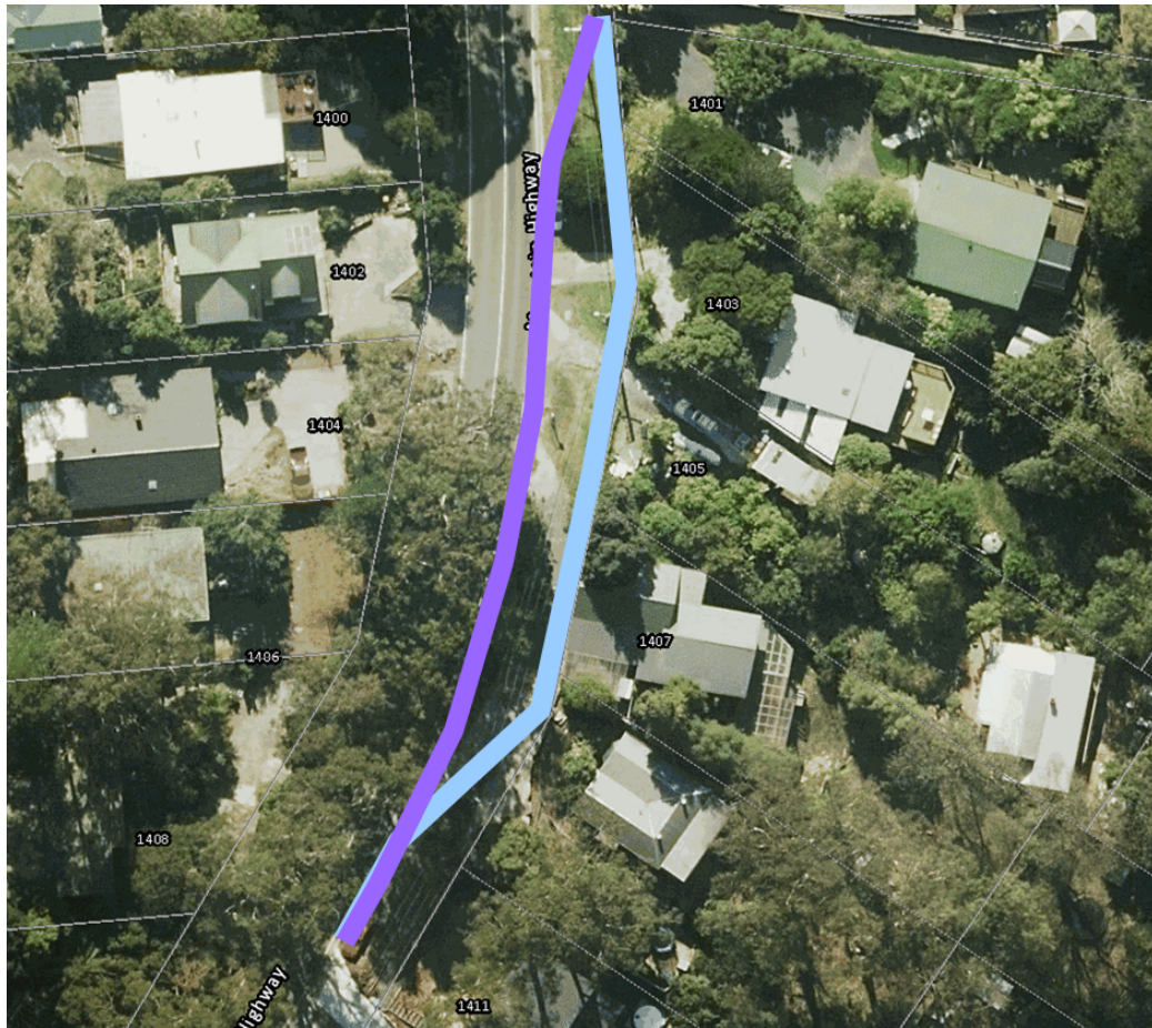
Figure 3: Proposed alignment variation – back of kerb (purple) versus along the property boundary (blue)
