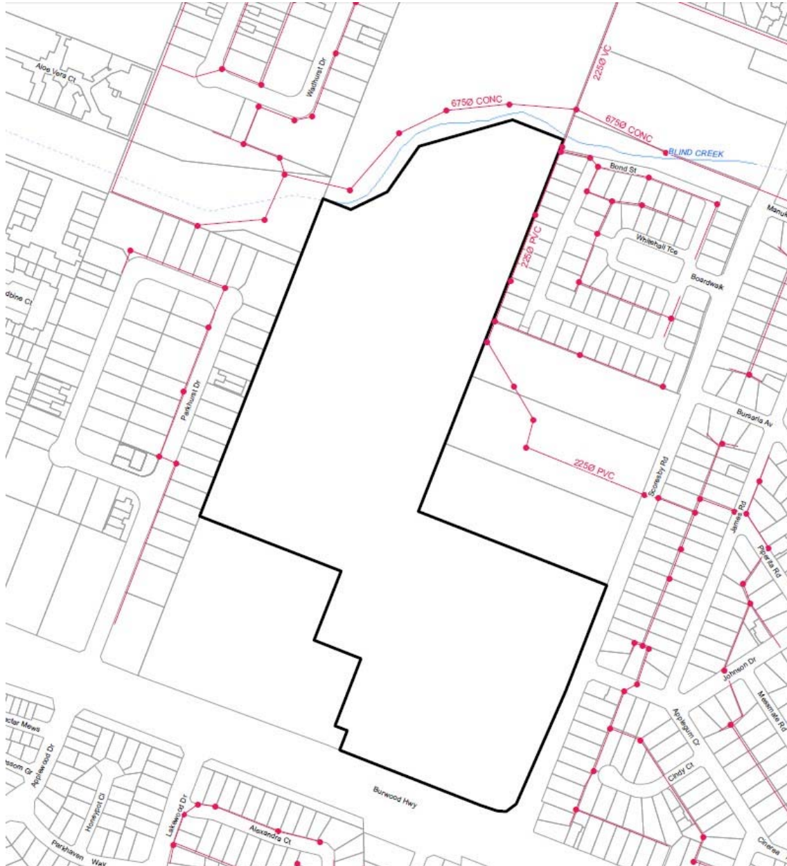
Figure 6: Existing Sewerage Infrastructure Adjoining 609-621 Burwood Hwy, Scoresby
