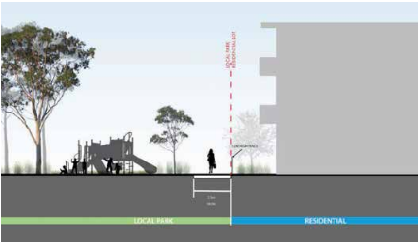
Figure 19. Local Park Interface Cross Section - Direct Lots
