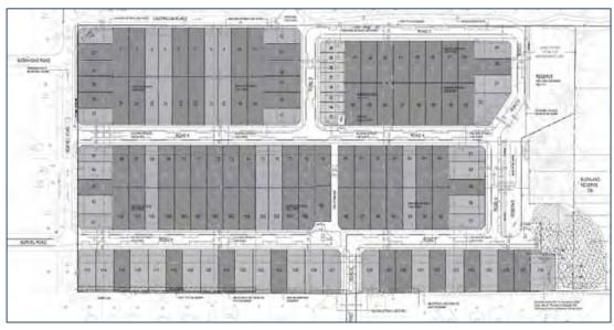
An internal road network of public roads will be constructed to provide access to most of the dwellings, although 21 dwellings will have direct access to either Norvel Road or Castricum Place and will not rely upon the internal road network.
