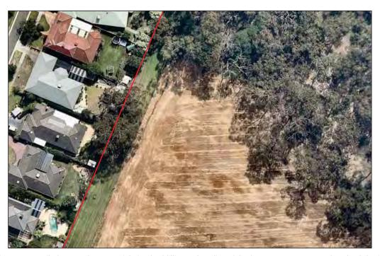
Figure 14: Detail of 20 March 2016 aerial after backfilling and grading of the former quarry, proposed wetlands basin area, western activity area boundary in red (Nearmap 2022)
